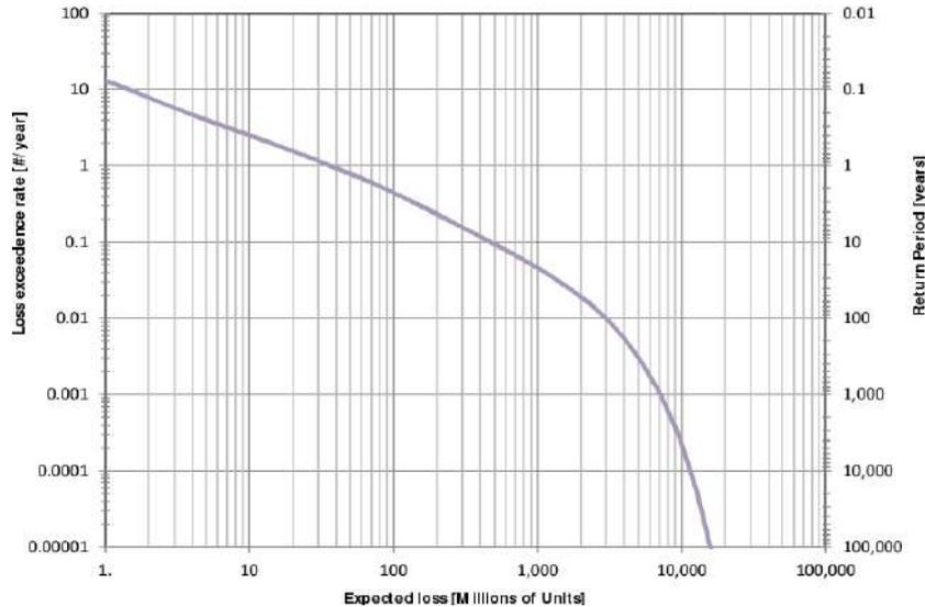
Figure 2.4: Loss exceedance curve. The left vertical axis shows the frequency while its inverse value on the right is the return period; the horizontal axis displays the expected loss (Velásquez et al. 2014).
