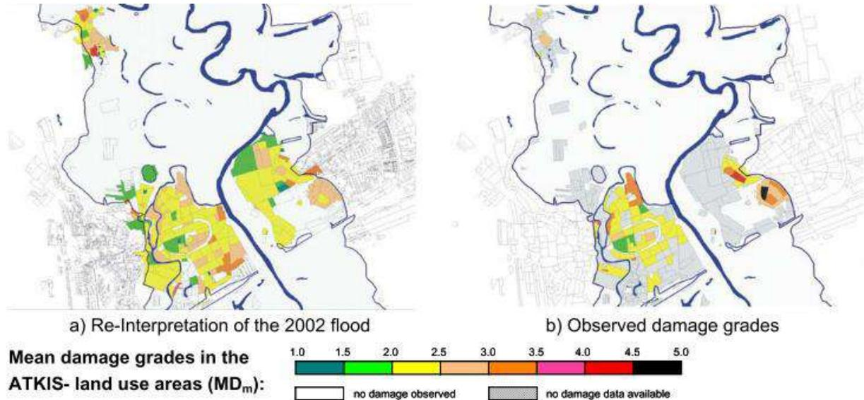
Figure 4.7: Comparison of calculated damages (left) and observed damages (right) using Schwarz and Maiwald (2008) tool
