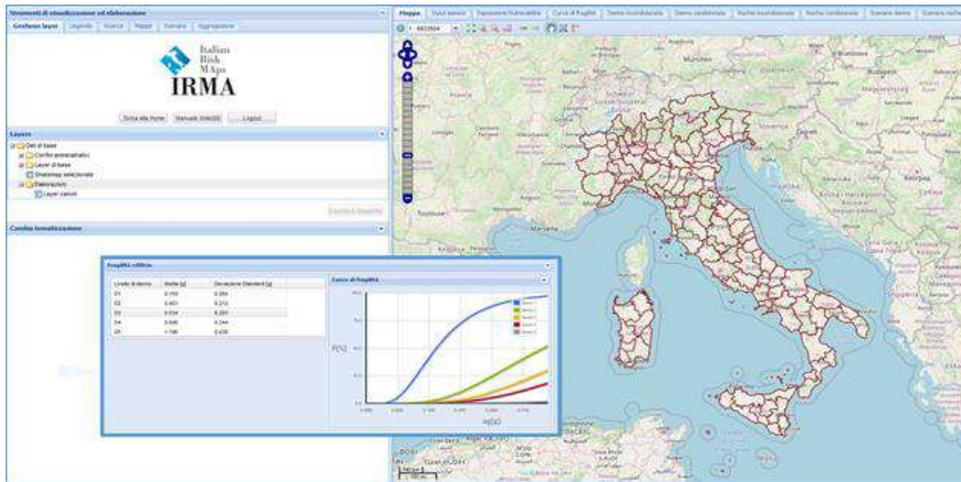
Figure 3.13: Homepage of IRMA platform and a set of fragility curves in the blue rectangle
