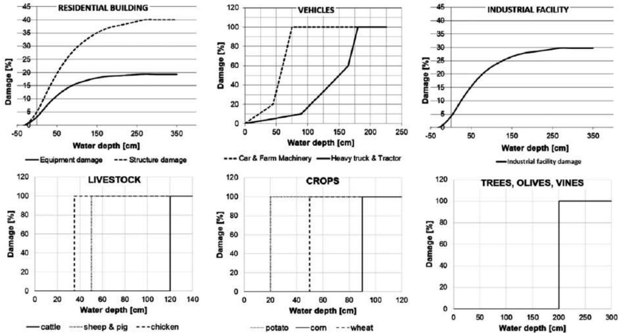
Figure 4.8: Depth-damage curves used in the NACER model (Vidmar et al., 2015).
