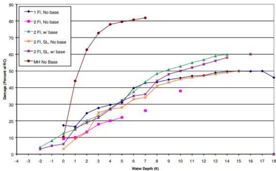
Figure 4.10: One set of depth-damage curves in HAZUM-MH model for residential buildings depending on the number of floors and presence of the basement (FEMA, 2014).
