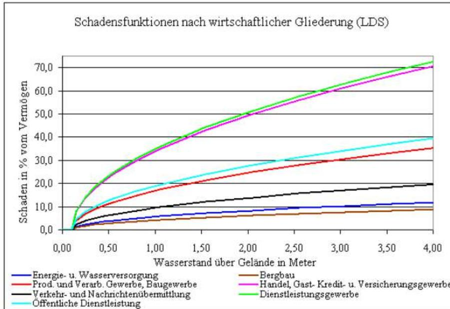
Figure 4.9: Depth-damage curves for different economic sectors used in Hydrotec model (Emschergenossenschaft and Hydrotec, 2004)
