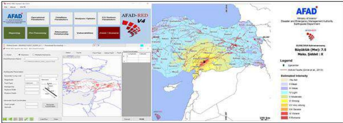
Figure 3.1 Screenshots of main and event/scenario menus of AFAD-RED (left side), an example output (right side)
