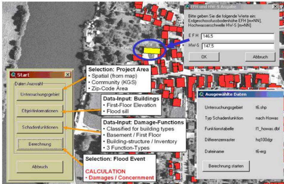
Figure 4.1: GUI of CEDIM model for flood risk assessment (adapted from Büchele et al., 2006)
