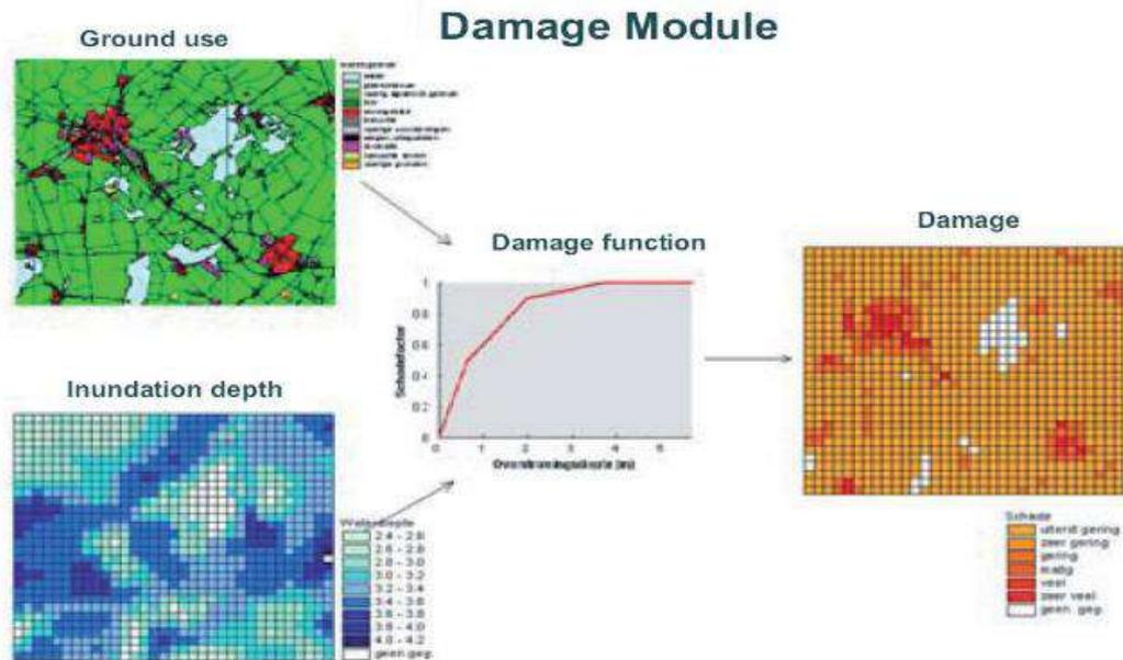
Figure 4.2: Schematic presentation of flood damage assessment in HIS-SSM model (Van Westen, 2005)
