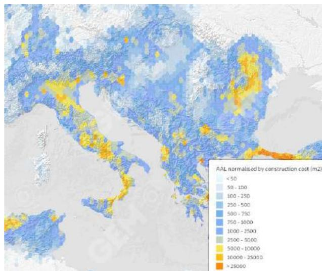
Figure 2.2: Example of a risk map that shows geographical distribution of the average annual loss due to earthquakes using colour codes (Silva et al. 2018, Global Seismic Risk Map v2018.1)
