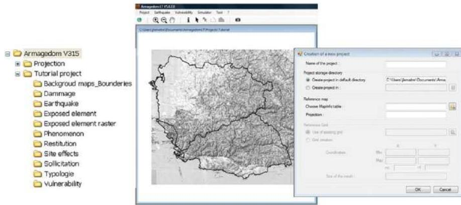
Figure 3.2: Project structure with the “catalog box” where data are loaded (left), main window (center), and the window for new project creation (right) (color figure available online) (Sedan et al. 2013)
