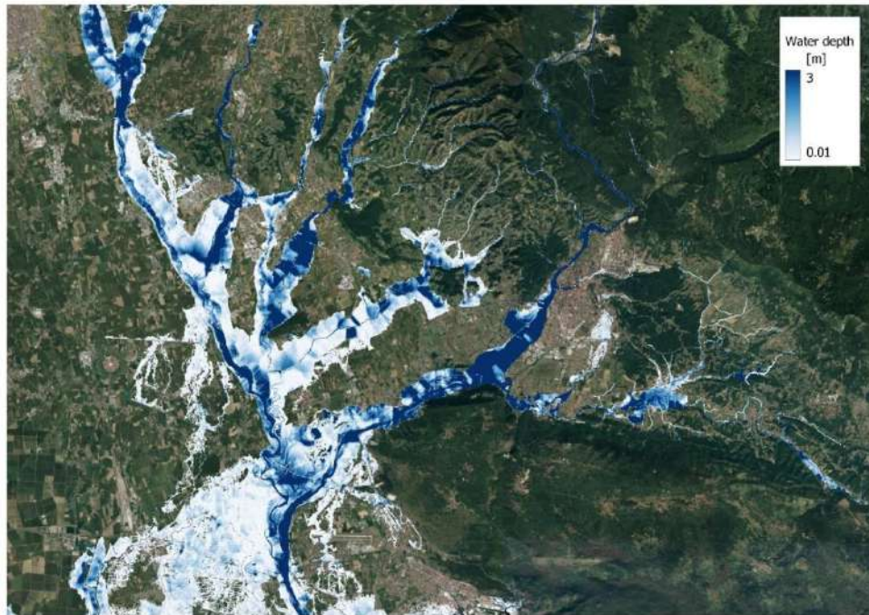
Figure 4.13: Example of harmonized flood hazard map in the Italy-Slovenia cross-border area (Isonzo river)
